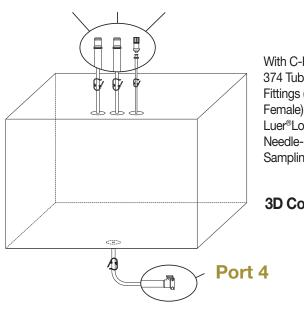
With C-Flex® Clear 374 Tubing, MPX Fittings (Male & Female), Female Luer®Lock with Needle-Free Sampling Port
