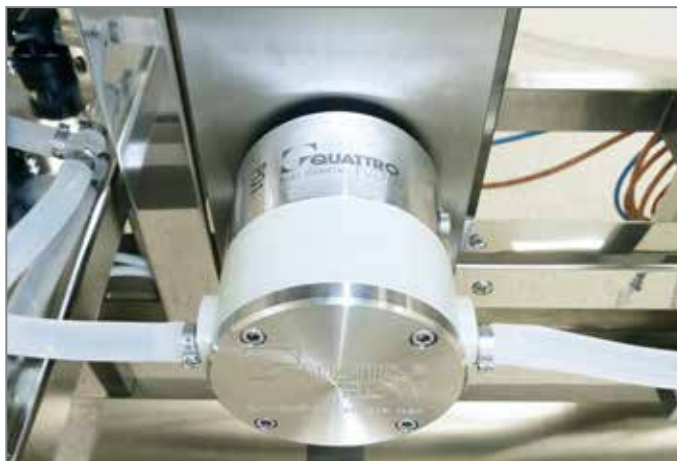
After its invention in 2000, quaternary diaphragm pump technology from Quattroflow™ quickly gained popularity as a low-pulse, low-shear option for the various unit operations that can be used in the manufacture of biopharmaceuticals.
